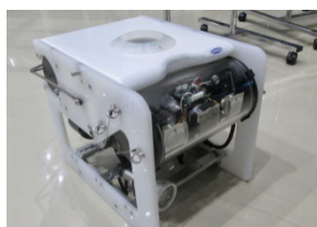
This underwater robot is equipped with a camera and light, which it uses to move around and conduct inspections inside the tank.
