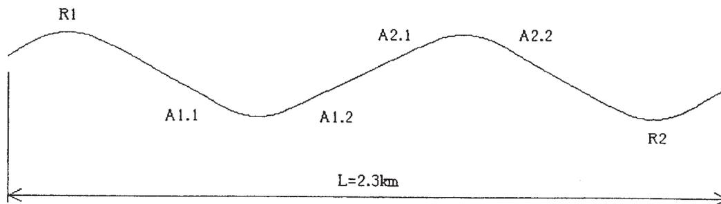
$$\begin{aligned} (1 \text{ km 当たり換算単曲線数}) &= (\text{換算単曲線数}) \div (\text{測線延長}) \\ &= \{ (\text{単曲線数}) + (\text{クロソイド曲線数}) \times 2 \} \div (\text{測線延長}) \\ &= (2 + 2 \times 2) \div 2.3 \\ &= 2.6 \quad 3 \text{ (箇所)} \end{aligned}$$
