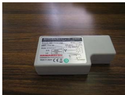
Figure17: High-dose CsI detector (Hamamatsu Photonics C12137).
