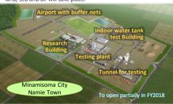
Construction of an Aerialdrone Area; Infrastructure inspection and disaster response area; On-water and under water robot area: and R&D infrastructure area is planned at a site extending 1,000 m east-west and 500 m north-south in Minamisoma City's Revitalization Industrial Park. There are also plans to construct a runway for long distance flight tests in Namie town's Tanashio Industrial Park.
