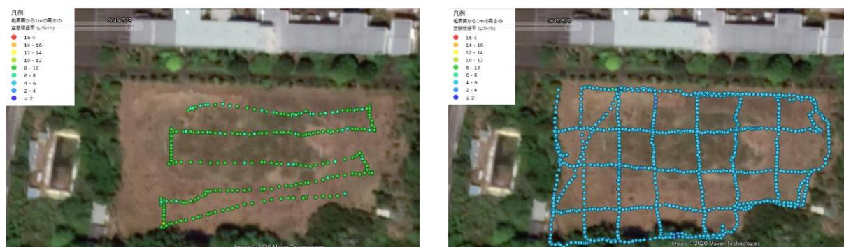
Fig. 5.2. Example of in-situ measurements (not-corrected raw data) performed in the area accessible both for backpack and UAV techniques: data points obtained with the UAV system (Geiger-Müller counter) flying at 10m altitude (on the left); data points obtained with backpack system (CsI spectrometer) walking throughout the area with the detector located at 1m altitude (on the right). Image: Fukushima Prefecture.
