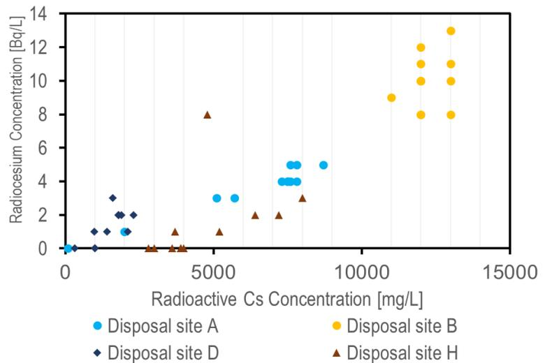
Figure 4. Correlation between radiocesium and chloride ion concentrations
